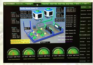
bearing compressors maintain their high efficiencies over their entire lifespan. At the heart of the system is the CPECS controller which operates the chillers, CHW pumps, CW pumps, and cooling tower fans, optimizing the entire chilled water plant at any point during the hotel's varying load conditions. The plant was commissioned in June 2013.
